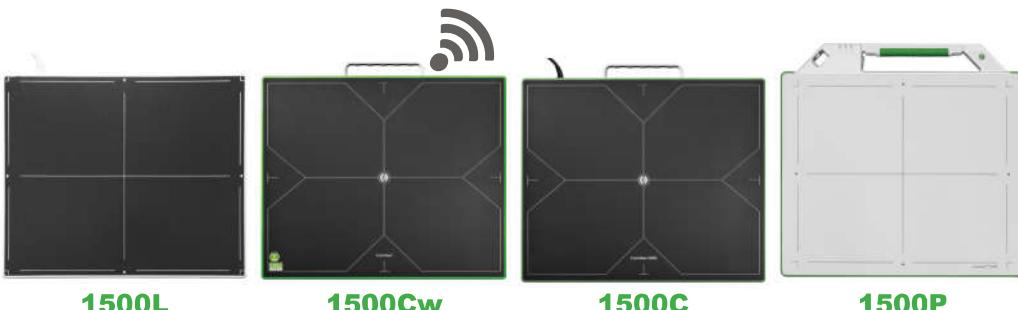
CareView® series X-ray flat panel detectors incorporate the proven technology of amorphous silicon. The amorphous silicon photodiode array and TFT underneath convert invisible X-ray photons into visible photons, and then into electric charges.
